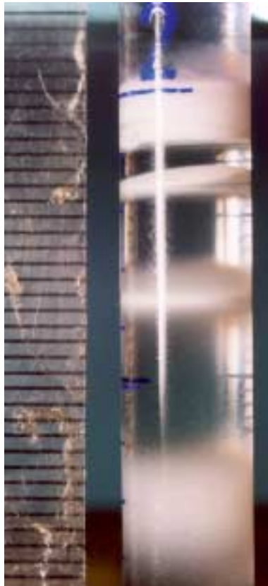
Figure 6: Mg(OH)_2 ring system grown in gelatin. The ruler shows 1mm markings.
