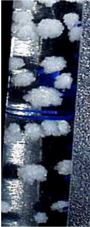
Figure 7: \text{Zn}(\text{OH})_2 spherulites growing in gelatin. Individual Spherulites are 2-3mm in diameter. This specimen was prepared with the protocol in Appendix C substituting Zn for Mg.
