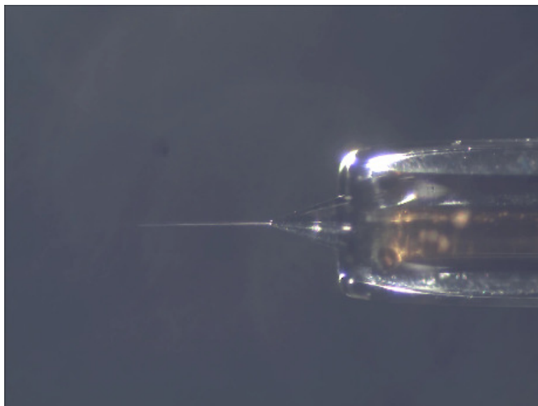
Figure 4.7: An example of a stable 20 \mu\text{m} agarose extrusion. The injector is mounted horizontally off-beam, so that visualization is improved. An air column of helium is used to stabilize the column.
