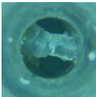
Figure 2.15: Viewing into the cell through a window port: trapped air bubbles in the sample chamber caused the silicone rubber sample-isolation piston to push into the sample chamber under pressure.
