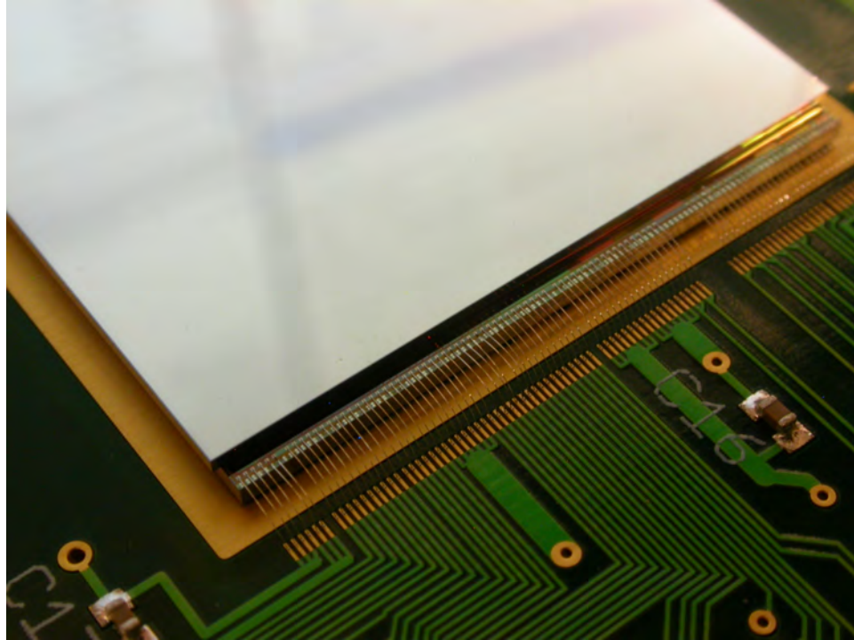
Figure 2.6: Photo of the CS-PAD hybridized ASIC wirebonded to support electronics. The wirebonds send biases and control signals to the ASIC, and also transmit readout signals from pixels to support electronics for processing and recording. The silicon sensor layer is about 20mm wide. (photograph by Mark W. Tate)
