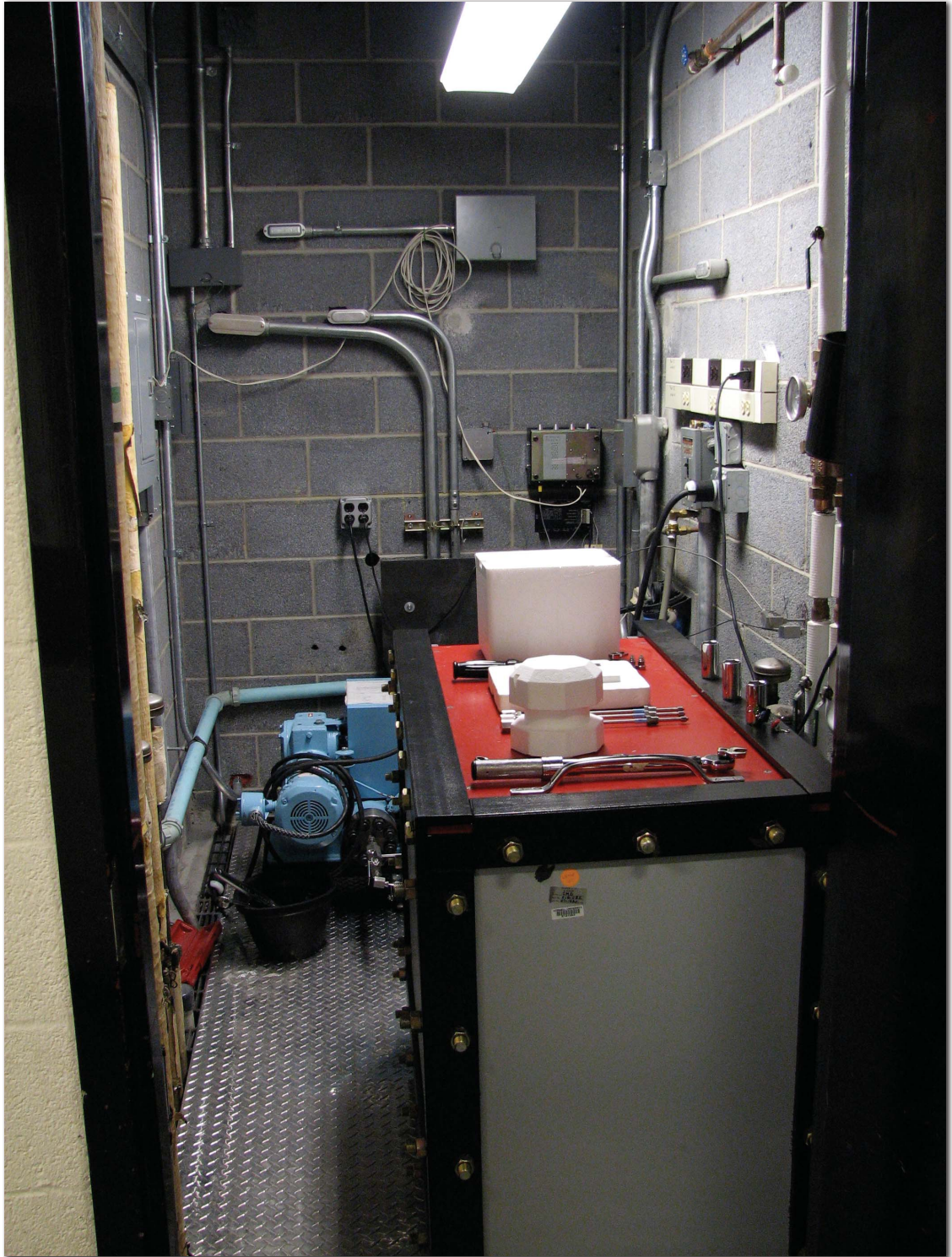
Figure 4.11: High-pressure cryocooling apparatus in its final assembled state.
