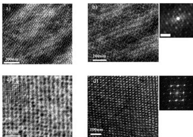
**Figure 2.** a) Dark-field TEM image of the as-made sample showing the continuous network structure. b) Dark-field image of the as-made sample showing network-struts. The inset shows the autocorrelation of the image; scale bar 100 nm. c) Dark-field image of the calcined sample. The black and the gray lines indicate the individual networks contained in the bicontinuous lattice. d) Bright-field image of the calcined sample. The inset shows the computed Fourier transform image.
