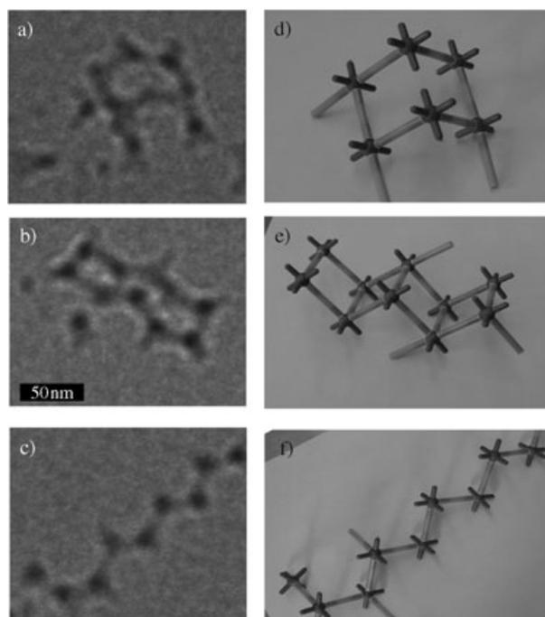
**Figure 3.** Bright-field TEMs of the broken network structure (a–c) dispersed in a toluene solution, and the corresponding projections from a bead–stick model (d–f). The scale bar in (b) is the same for all TEMs. The distance measured between the nodes are in accord with the expected value from SAXS and TEM measurements.
