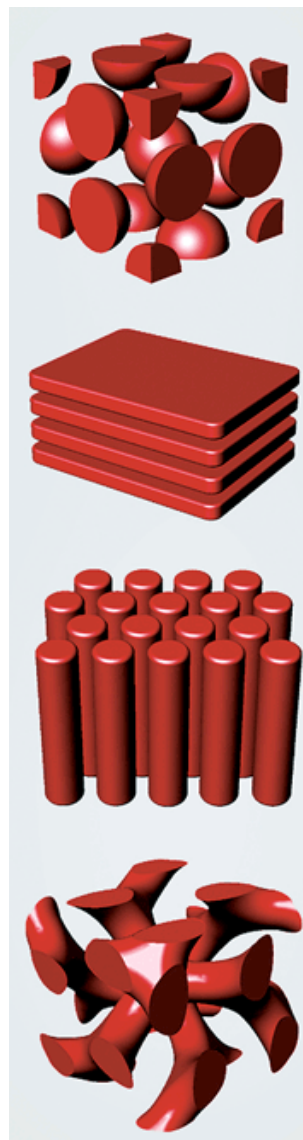
MESOPHASE MORPHING Novel hybrid molecules assemble into (from top) cubic micelles, layered structures, cylindrical columns, and continuous cubic structures.
