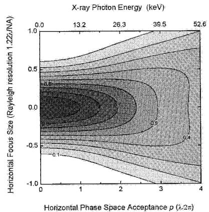
Figure 2. Focal spot size of a focusing optic versus the accepted phase space area in units of  $\lambda/2\pi$ . Given the fixed ERL emittance of 0.015 nm-rad, it shows that full undulator radiation within the central cone can be accepted up to 13 keV without significant degradation of resolution for SXM applications.
