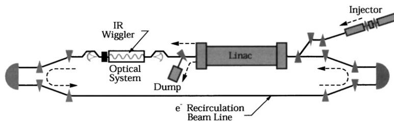
Fig. 2. Jefferson Laboratory IR-FEL. The Jefferson Laboratory IR-FEL is also a single-pass machine. Electrons from the injector are brought up to energy in the linac and then pass through a wiggler magnet to create the IR. Mirrors at the ends of the wiggler magnet intensify the IR beam. The electrons circulate around the rest of the lattice before their energy is recovered in another pass through the linac, after which they are sent to the dump. (Source: Jefferson Laboratory web site).
