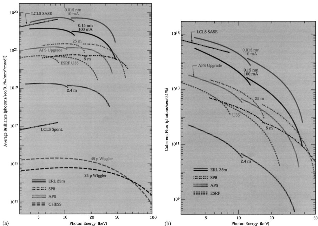
Fig. 3. Expected average brilliance (a) and coherent flux (b) for an ERL based on the Cornell/Jefferson Laboratory design described in [http://erl.chess.cornell.edu/Papers/ERL\\_Study.pdf](http://erl.chess.cornell.edu/Papers/ERL_Study.pdf). The ERL may be operated either in a high-flux mode (100 mA, 0.15 nm emittance) or, by reducing the photocathode current to decrease the photoinjector emittance, in a lower flux mode with very high brilliance (10 mA, 0.015 nm emittance).
