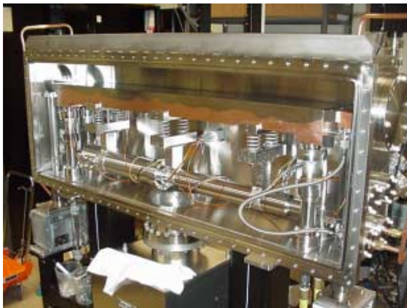
Figure 1. CHES F-line white-beam mirror in its ultra-high-vacuum vessel. It consists of a flat Glidcop substrate with rhodium coating, a variable-force U-bender, and a system of springs for gravity compensation.
